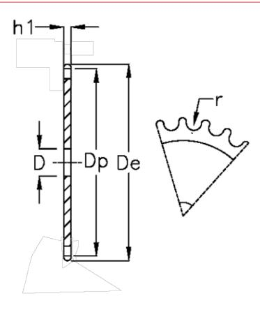
C = 6 D = 30 De = 313 Dp = 292.55 For chain size = 2 x 1 1/4 For chain type = 32 B-1 h1 = 29.4 Solution Number of teeth = 18
